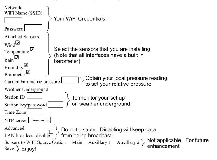
9. Once the information is entered the instrument interface will connect the sensor interface and the instruments will start operating. The Maximum interface LED will change to both green.
