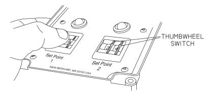
The thumbwheel switch directly below each LED controls the yellow or red warning lights. Adjust the speed that you want to set off the yellow or red light by pushing the adjustment lever on the thumbwheel switch to the desired wind speed. Once the wind speed reaches the level set on the thumbwheel switch, the yellow or red light will turn on and activate the relay. When both lights are activated, the buzzer will sound.
