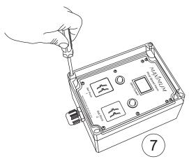
Remove the clear cover by removing the corner screws
