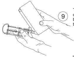
Tilt the enclosure forward until the circuit board drops out. (The circuit board will not drop out completely if the optional latching switch is installed.)
