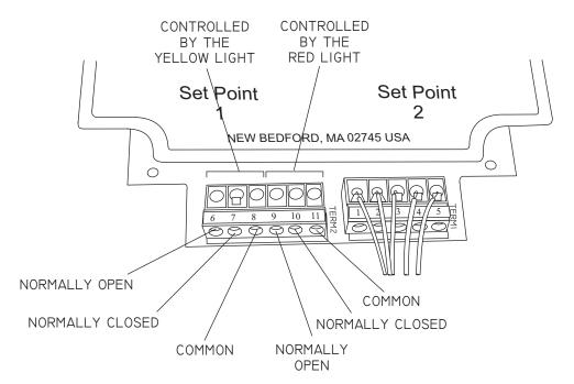
The relays are SPDT. If you are looking at the relay terminal block, the yellow light controls terminals 6, 7, and 8. Prior to reaching the set point, terminals 7 and 8 are normally closed and terminals 6 and 8 are normally open. The red light controls terminals 9, 10, and 11. Prior to reaching the set point, terminals 10 and 11 are normally closed and terminals 9 and 11 are normally open.
