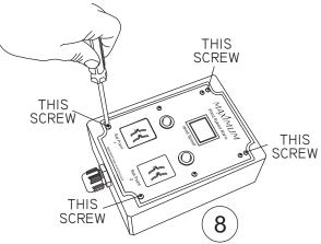
Remove the circuit board from the plastic enclosure by removing the screws on each corner.
