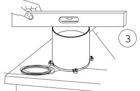
If the collector is not mounted absolutely level your readings will be incorrect.
