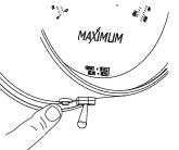
A. Pushing the select switch to the left and holding the push button switch for six seconds erases "Current".
