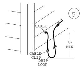
Run the wire into the house using insulated cable clips. Form a drip loop where the wire enters the house and caulk the feed thru hole when done
