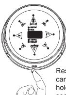
To reset all the stored funcions at once, select the "Present" function by moving the switch to the right and releasing until the "Present" light is illuminated. Then hold the switch to the left until the display blanks out (about six seconds). The unit will then perform a self-test and return to normal operation.
