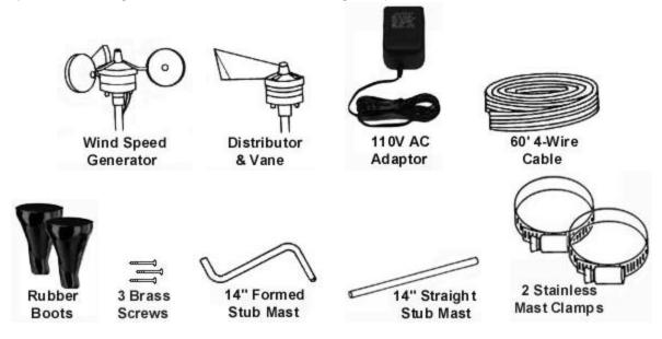
**Rooftop sensors:** To insure a clear unobstructed path for the wind to the sensors, they should be mounted on some type of antenna mast at least 810' above the highest object on your roof. Remember, your roof is also an obstruction and it usually requires at least 8' of height to avoid the turbulence it creates.
