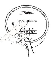
Disconnect the sensor wires from the back of the meter.
