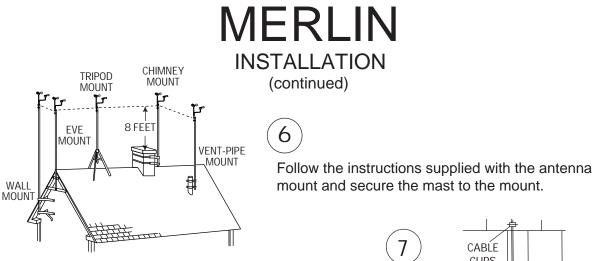
Secure the wire to the building using cable clips (do not use regular staples). Form a drip loop where the wires enter the hole drilled through the exterior wall. Caulk the hole when done.
