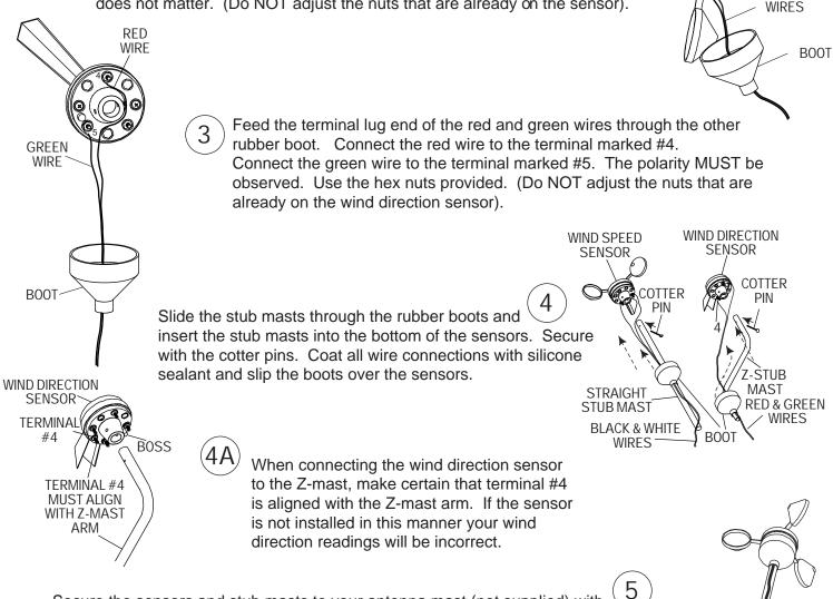
Secure the sensors and stub masts to your antenna mast (not supplied) with the two hose clamps. **Align the wind-direction Z-mast arm to true North**. Radio Shack and similar stores have a selection of tall masts and roof mounting brackets. Choose a mount that best suits your location and provides at least eight feet of vertical clearance above objects on the roof.
