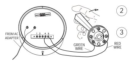
Remove the sensor from the roof and connect it to the indicator with short pieces of wire.
