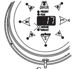
To auto-sequence through all of the functions, hold the switch to the right for at least three seconds. You will see each function light stay on and the corresponding information displayed for approximately four seconds. MERLIN will then move to the next function automatically.
