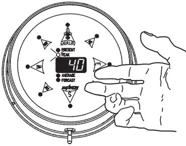
With the switch in the center (resting) position, MERLIN will display the information indicated by the illuminated function (Present, Peak, Average, or Forecast).
