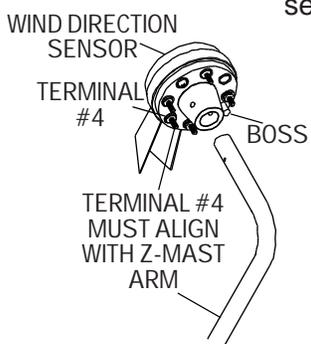
Slide the stub masts through the rubber boots and insert the stub masts into the bottom of the sensors. Secure with the cotter pins. Coat all wire connections with silicone sealant and slip the boots over the sensors.
