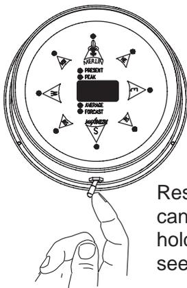
Resetting the Peak, Average and Forecast functions Individually can be done by toggling to the function that you wish to reset. Then hold the switch to the left for at least 6 seconds. At that point you will see the display reset itself.
