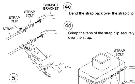
Feed the stainless straps around the chimney without twisting them. Repeat steps 4a-4d to secure the loose strap ends to the brackets. Cut off any excess material once secure. Brackets should be at least 18" apart for proper mast support.
