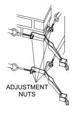
Tighten the stainless steel straps with the adjustment nuts at the ends of the strap bolts. Make sure straps are centered on bricks and not mortar.
