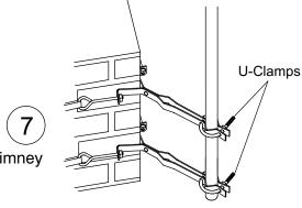
Insert the bottom of the mast into the chimney brackets and secure with the U-clamps.
