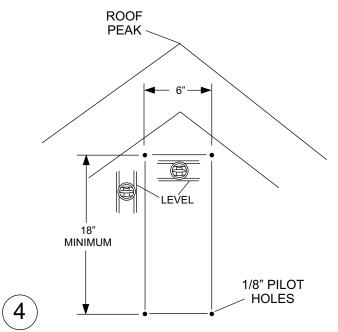
Drill two 1/8" level pilot holes 6" apart for each bracket. Brackets must be separated from each other by at least 18" for mast stability. Both brackets must be aligned vertically for the mast to be straight when installed.
