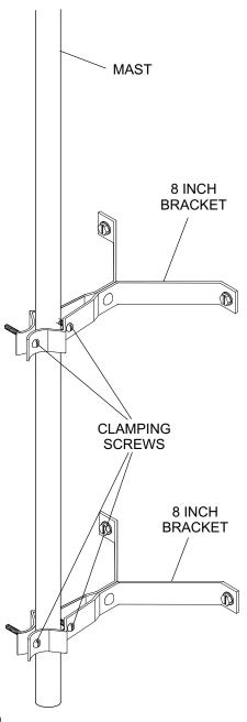
6 Slip mast into brackets and tighten with the clamping screws.
