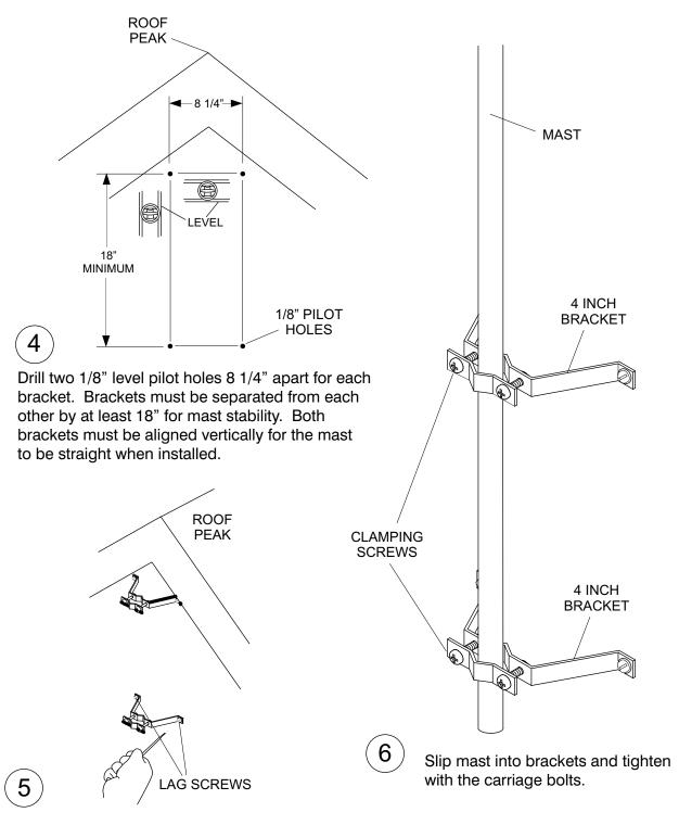
Secure the brackets with the lag screws
