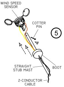
Slide the straight stub mast through the black rubber boot and insert it into the Wind Speed Sensor, securing it with the supplied stainless steel cotter pin. Once the final installation is made and proper function is verified, coat all the wire connections with a silicone sealant designed for electrical connections (not supplied). Slip the boot over the base of the sensor.
