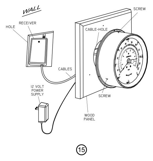
Mount the brass instrument meter directly over the cable hole that is also used to route power to the instrument. For the cleanest installation, we recommend making a hole in the wall large enough to insert the wireless receiver. We also recommend mounting the brass meter to one of our pre-drilled mounting panels.
