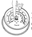
Turning the knob counter-clockwise will eventually contact the gust register. The Gust Register should not be set under 15 MPH - this gives the needle room to operate at low speeds. If the Gust Register is set below 15 MPH turn the knob clockwise until the needle registers greater than 15 MPH.
