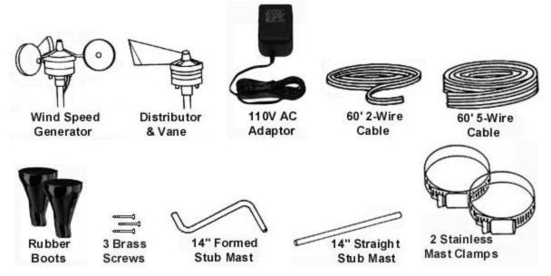
**Rooftop sensors:** To insure a clear unobstructed path for the wind to the sensors, they should be mounted on some type of antenna mast at least 810' above the highest object on your roof. Remember, your roof is also an obstruction and it usually requires at least 8' of height to avoid the turbulence it creates.
