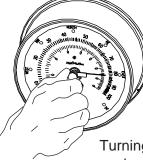
Turning the knob counter-clockwise will eventually contact the gust register. The Gust Register should not be set under 15 MPH - this gives the needle room to operate at low speeds. If the Gust Register is set below
