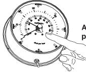
After setting the Gust Register turn the knob clockwise until the reset arm is parked near the six o'clock position. Failure to do so may damage your meter.
