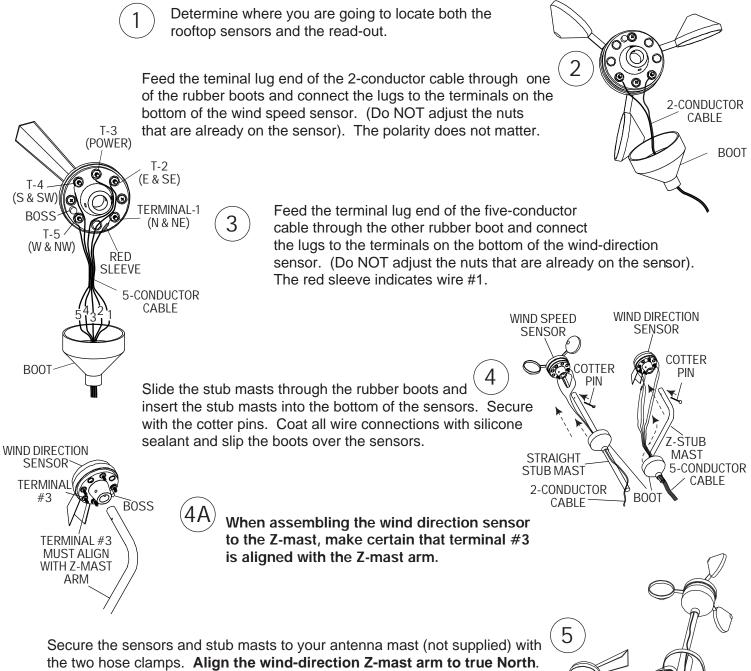
the two hose clamps. Align the wind-direction Z-mast arm to true North Radio Shack and similar stores have a selection of tall masts and roof mounting brackets. Choose a mount that best suits your location and provides at least eight feet of vertical clearance above objects on the roof.
