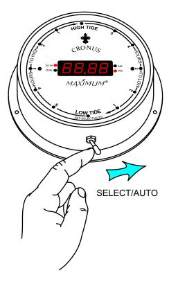
Pushing the switch to the right "SELECT/AUTO" and allowing it to return to the middle will toggle Cronus between time and date. This will be indicated by the illuminated function light (AM, PM, 24 hr or, Date).
