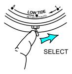
Cronus uses the same basic setting method for all values. The value being set will be flashing. Pressing the switch to the left "SET" will select different items to be set. Pressing the switch to the right, "SELECT", will change the flashing value. When no values are flashing, and the "seconds"indicator is flashing twice per second. pressing the switch to left "SET" will end the setting operation.
