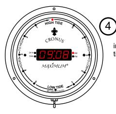
When Cronus starts up, it checks the tide time stored in the battery backed up memory. If it finds that the tide in memory is prior to the current time, it advances the tide time to the next tide in the future.
