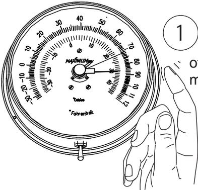
1 Before reading your thermometer, you should lightly tap the case with your finger. A TAP change of 1-2 degrees is a common occurrence with any slow moving precision meter movement.
