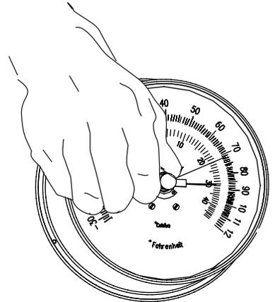
2 The trend register needle can be set by turning the center knob on the indicator dial.
