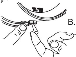
B. Pushing the select switch to the right and holding the push button switch for six seconds erases "Total".
