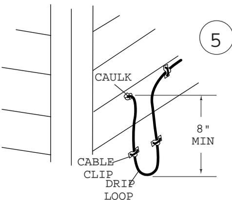
5 Run the wire into the house using insulated cable clips. Form a drip loop where the wire enters the house and caulk the feed thru hole when done
