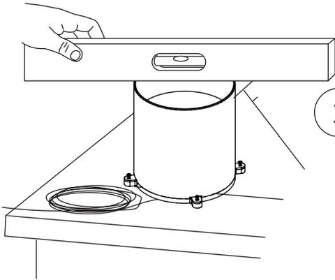
3 If the collector is not mounted absolutely level your readings will be incorrect.
