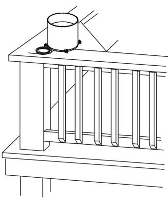
1 Select a level surface in an open area above ground to mount the collector. Some examples would be a deck or tree stump.
