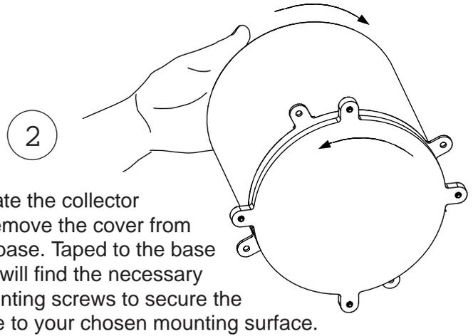
2 Rotate the collector to remove the cover from the base. Taped to the base you will find the necessary mounting screws to secure the base to your chosen mounting surface.
